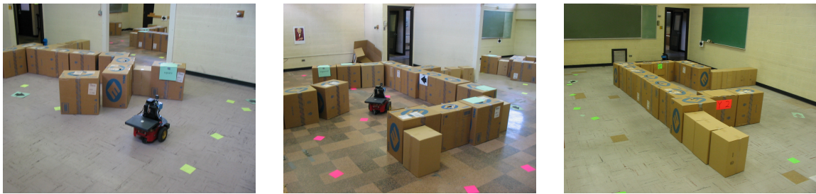
Figure 5.1: Some pictures of the space we used for real-world experiments. The picture on the left shows the robot halfway through the first room of the test environment. The middle picture shows the second room, and the right picture shows the last room and the hallway between the second and third rooms.
